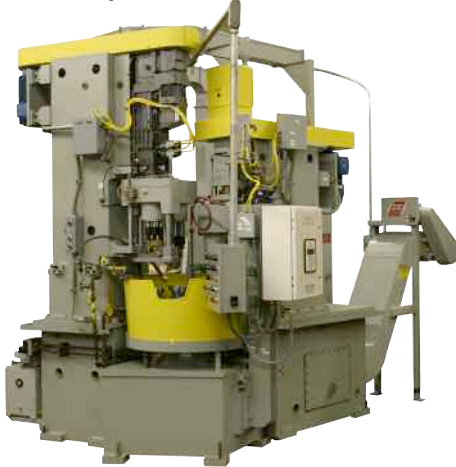
Rockford Six Station Dial Index machine produces finished, validated parts
